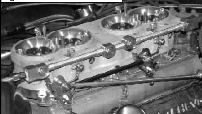
Figure 5 - Fuel Rail Installed
